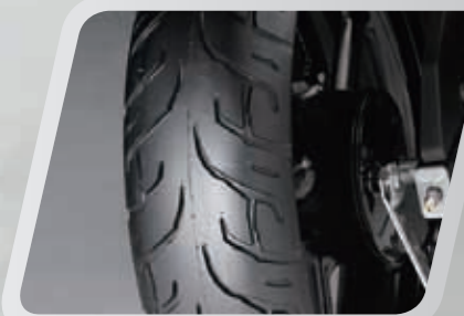
India's First 140/60-17 size Radial Tyre (Rear) Widest radial tyre for solid control & grip even on bumpy and wet roads.
